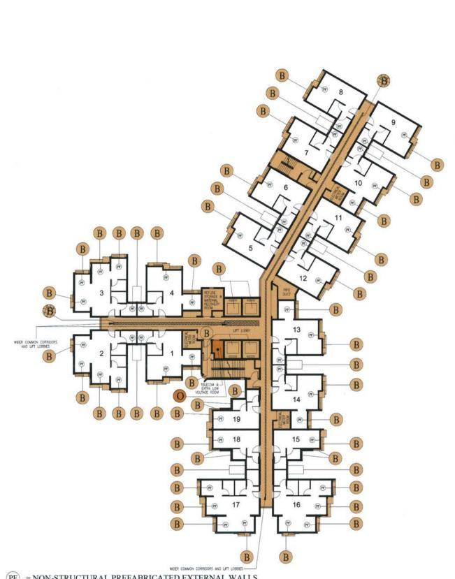
(PF) = NON-STRUCTURAL PREFABRICATED EXTERNAL WALLS
